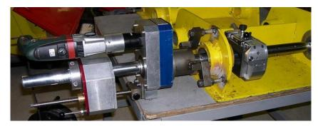
This attachment needs no other motor than the one of the portable boring bar.
